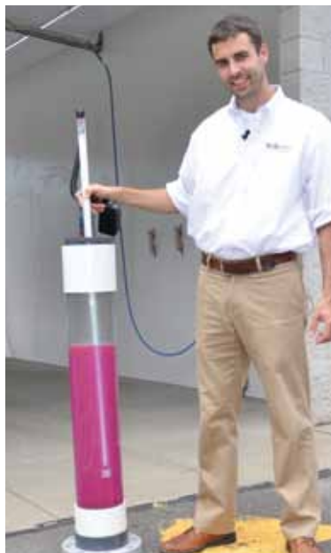
LED Tube fully lit and submerged in soapy water solution.
